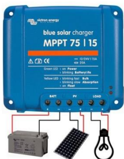
Figure 4: Power connections
